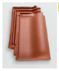
Gauge: 36.0 - 36.6 cm Req. per m<sup>2</sup>: from12.5 tiles Standard roof pitch 16° Min. roof pitch 10° Hail resistance class 4
