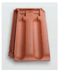
Gauge class 38.5 cm Gauge: 37.7 – 39.7 cm Req. per m<sup>2</sup>: from 9.8 tiles Standard roof pitch 22° Min. roof pitch 10° Hail resistance class 4
