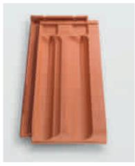
Gauge<sup>1)</sup>: 32.6 – 34.6 cm Gauge<sup>2)</sup>: 32.6 – 33.8 cm Req. per m<sup>2</sup>: from 15.0 tiles Standard roof pitch 30° Min. roof pitch 10° (laid in straight bond or cross-bond) Hail resistance class 4
