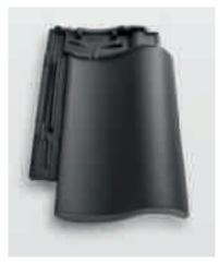
Gauge: 32.5 – 35.5 cm Req. per m<sup>2</sup>: from 11.5 tiles Standard roof pitch 20° Min. roof pitch 10° Hail resistance class 4
