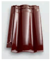
Gauge class 38.5 cm Gauge: 37.7 – 39.7 cm Req. per m<sup>2</sup>: from 9.9 tiles Standard roof pitch 22° Min. roof pitch 10° Hail resistance class 4
