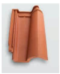
Gauge class 34.0 cm Gauge: 33.7 – 34.2 cm Req. per m<sup>2</sup>: approx. 14.5 tiles Standard roof pitch 22° Min. roof pitch 10° Hail resistance class 4
