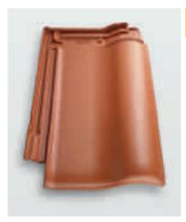
Gauge: 40.5 – 43.5 cm Req. per m<sup>2</sup>: from 7.4 tiles Standard roof pitch 20° Min. roof pitch 10° Hail resistance class 5
