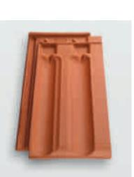
Gauge class 34.0 cm Gauge: 33.8 - 35.1 cm Req. per m<sup>2</sup>: approx. 12.5 tiles Standard roof pitch 25° (laid in cross-bond, 5° higher for straight bond) Min. roof pitch 10° Hail resistance class 4
