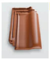
Gauge: 33.8 – 34.3 cm Req. per m<sup>2</sup>: approx. 14.5 tiles Standard roof pitch 20° Min. roof pitch 10° Hail resistance class 4
